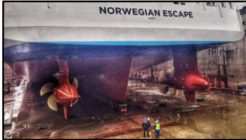
Image 16. VLCS Norwegian Bliss twin azipod propulsion (sister ship Norwegian Escape shown)
